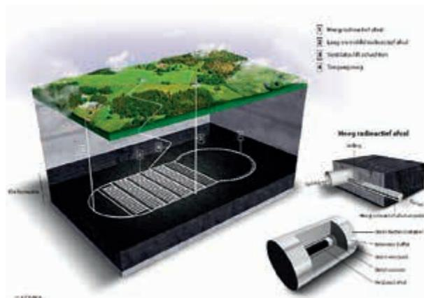
Figure E.3 Artist's impression of the disposal concept in Boom clay (OPERA).
